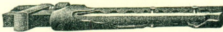
SECTION OF HANDLE SHOWING INTERNAL SUPPORT OF STEEL SHELL
